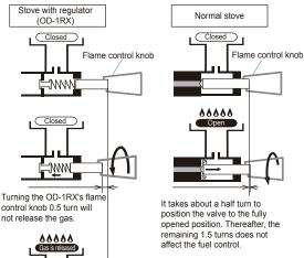
The flame control knob must be turned at least 1-1.5 turns in order to release the gas.
