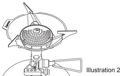
2. Set one a pot support. Then, place a □ or raised area of the Micro Windscreen on the pot support as shown in illustration 1. Set the remaining two pot supports. The rest of the □s, or raised areas on the windscreen, must be directly placed on the remaining pot supports.
